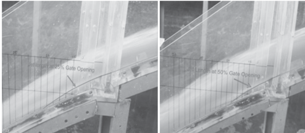
Figure 9. Measurement of Jet length at reservoir level of 1620 masl and at gate opening of 25% & 50%
